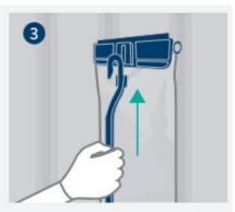
Fit the hook on the back (non-printed side) by pushing it up into the slot.
