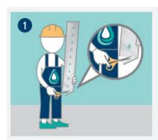
Activate the Absorbag by opening the transparent outer plastic packing and taking out the Absorbag. Be careful not to cut into the Absorgel.
